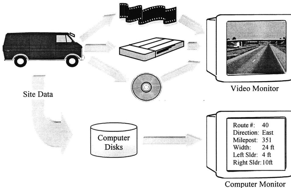
Figure 1 – The Existing Photo-logging System Data Flow
