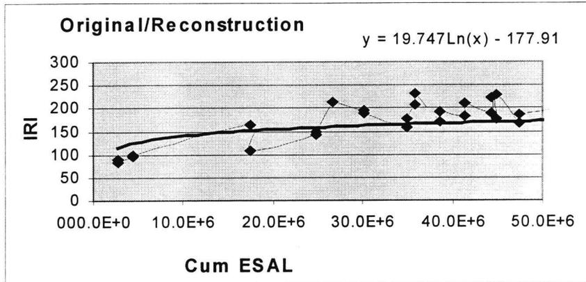
**Figure 3 – IRI Performance Curve (Original Pavement)**
