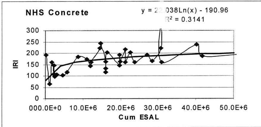
**Figure 5 – IRI Performance Curve (Concrete, FNCLA All)**
