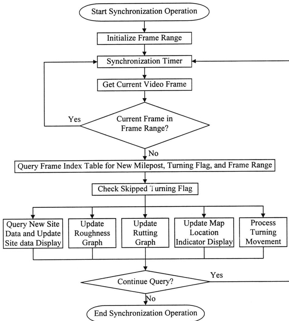
Figure 4 – The Synchronization Process Flow Chart
