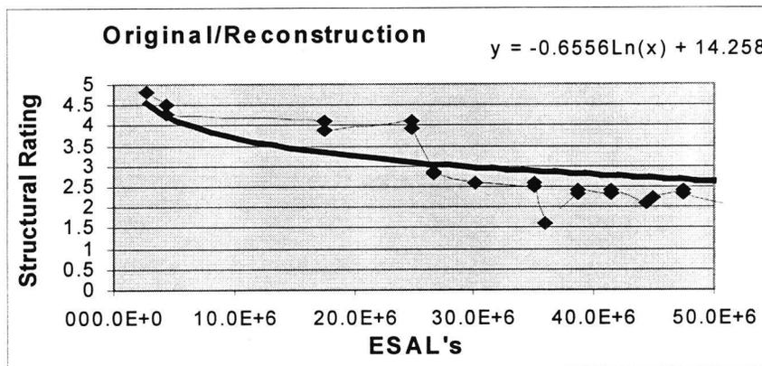
**Figure 4 – SRI Performance Curve (Original Pavement)**
