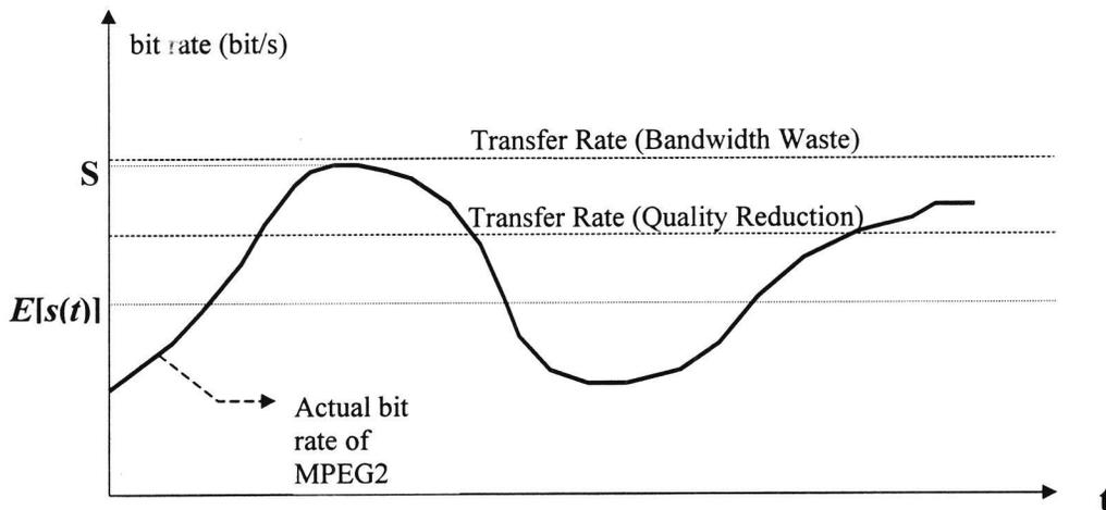
**Figure 8 – Buffering Scheme for Video Stream Playback**
