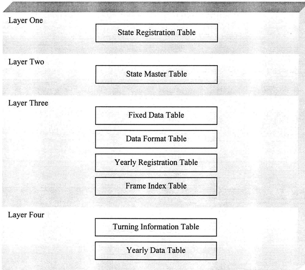
Figure 5 – The Layered Database Structure For MMHIS
